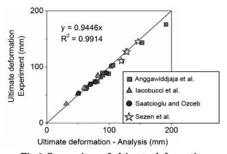
Fig.9 Comparison of ultimate deformation
