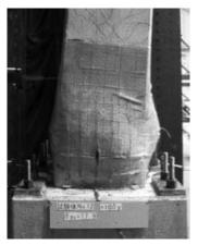
Fig.12 PET jacket performance after large plastic deformation
