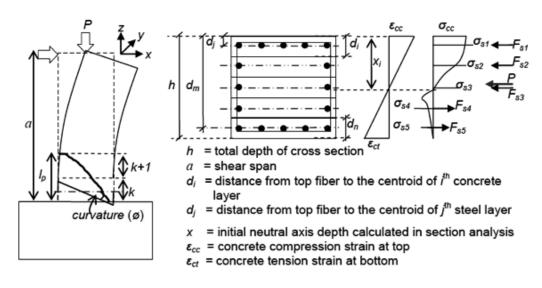
Fig.2 Section analysis for flexure model
