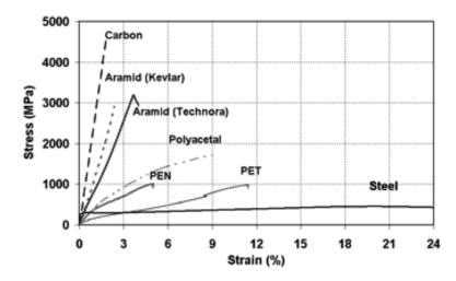
Fig. 10 Comparison of stress - strain relationships of various structural materials
