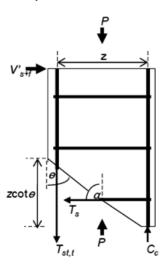
Fig.5 Effect of shear cracking on flexure deformation
