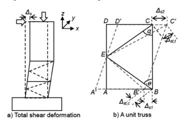
Fig.6 Shear deformation model
