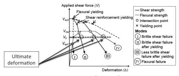
Fig.1 Ultimate deformation on load (shear force) – deformation curve
