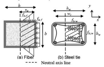
Fig.3 Confinement effects by jacket and tie reinforcement
