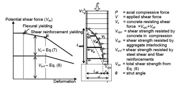
Fig.4 Shear strength model
